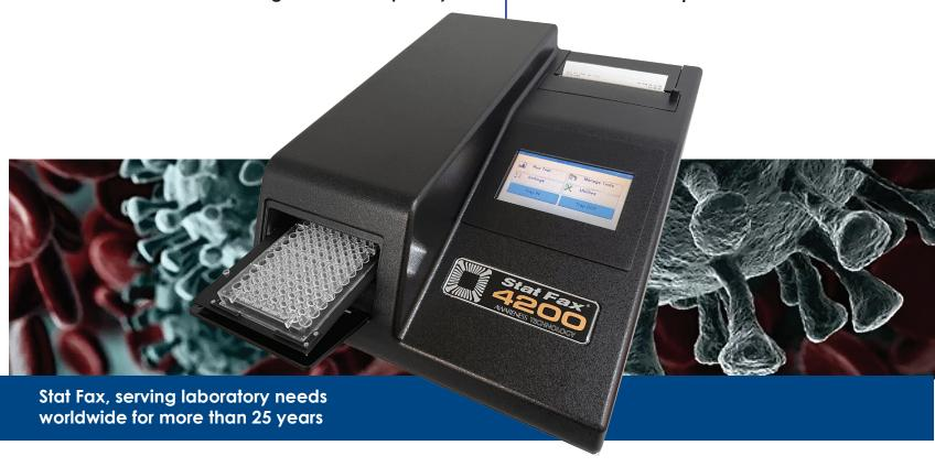
The Stat Fax® 4200 is a compact, standalone 8-channel microplate reader. Featuring an intuitive touch-screen interface, rapid reading capability of 96 wells, superb optics, six filters with a filter range of 405-700 nm, maintenance-free design.
